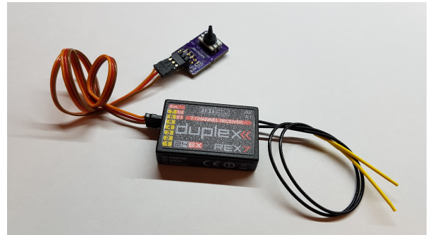
SB-PSENSE connected to Jeti receiver
