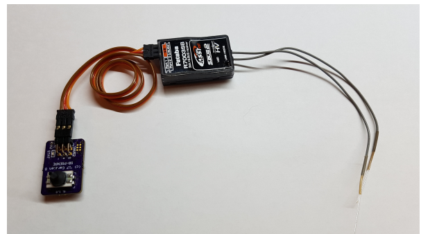
SB-PSENSE connected to Futaba SBUS2 receiver
